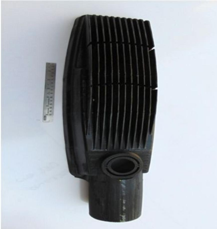
Prototype of Greenstar's design printed by ProtoCentre 3D printer.
